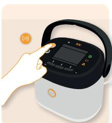
1. If the device is on and therapy is being delivered, pause it by pressing .
